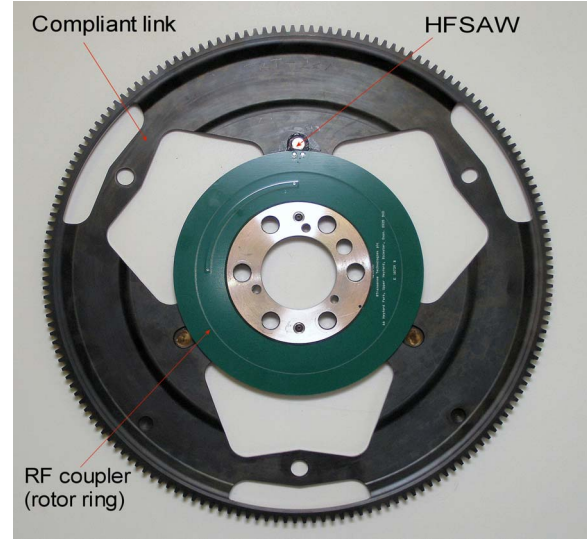
Figure 2. Flexplate with a single sensing element and a rotor ring of the RF coupler
